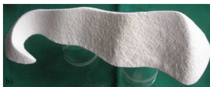
Model of the embankment with a natural slope: a) in AutoCAD, b) a real pile of granular material
