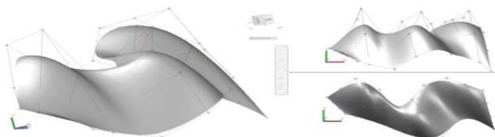
Fig. 2 Geometric Construction of NURBS object consisting of a mesh and control points called nodes. Development in AutoCAD 2011.
