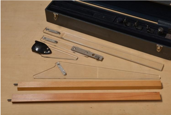
Fig. 1. Perspectograph PREMA, made in Czechoslovakia, the 50s of the last century
